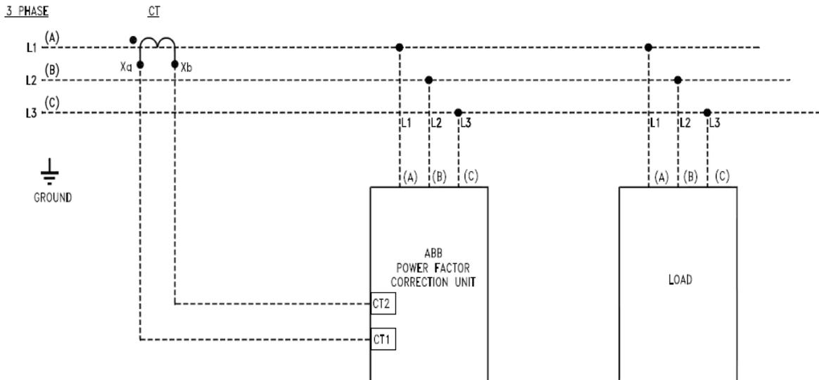
Figure 9: Single CT connection example
