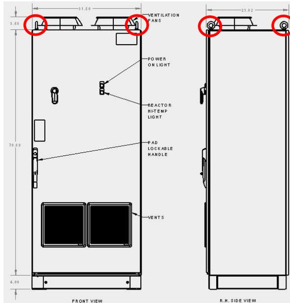
Figure 1: Lifting eyes
