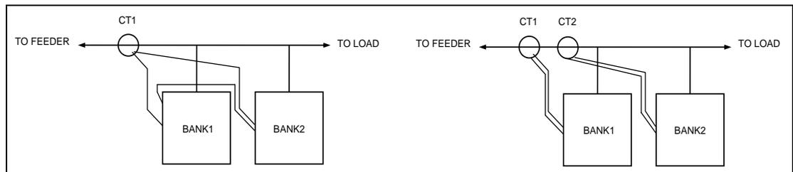
Figure 11: Connection of several capacitor banks in parallel
